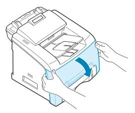
2 Pull the toner cartridge out and gently roll the cartridge 5 or 6 times to distribute the toner evenly inside the cartridge.
